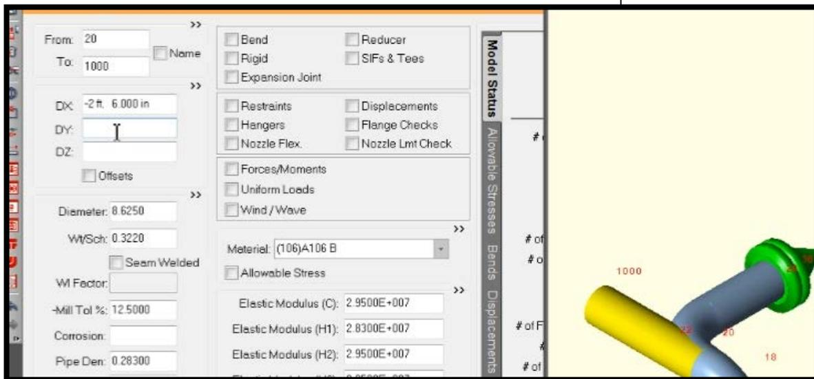
The system added the pipe at the same diameter, and when modeling a dummy leg it's common to make it a smaller diameter, typically smaller by one or two sizes.
