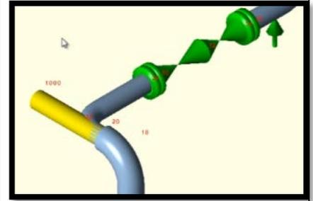
11. When we changed the size to 6", the system set all the following pipes to that same diameter.
