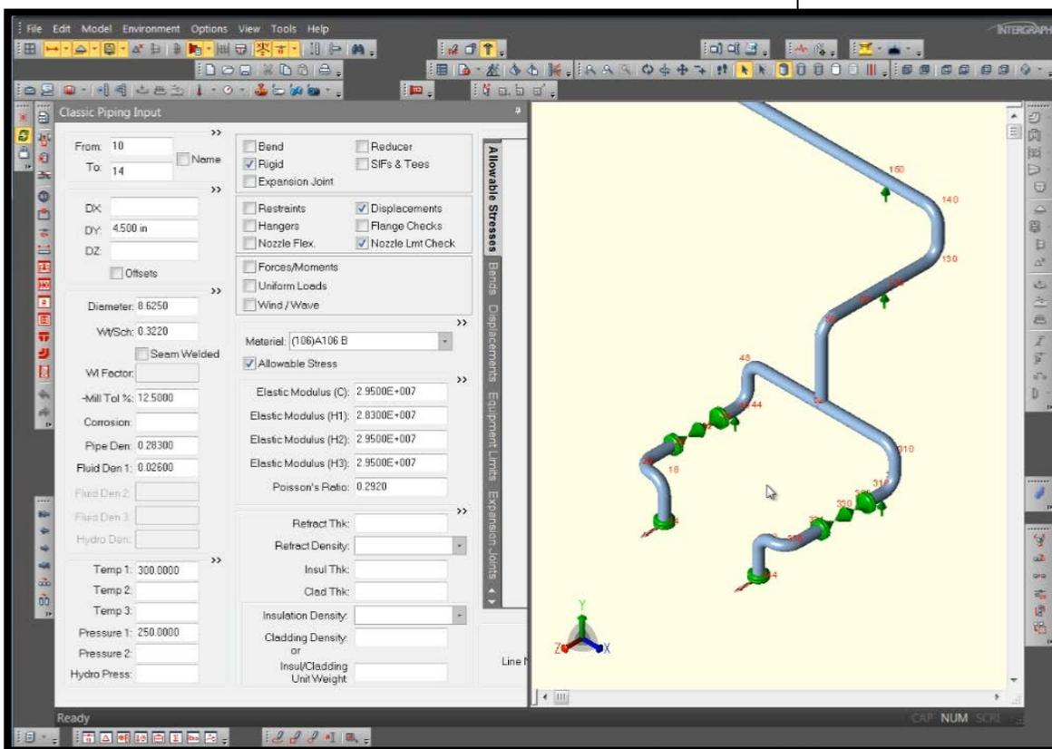
That results in a moment around the X axis that is greater than what's allowed in the nozzle limit checks. But this gives us an excellent opportunity to model a dummy leg in this line to reduce that moment. In the process we'll learn some new features and techniques in CAESAR II.
